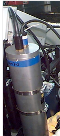
Figure 16. (A) Flight tracks for aircraft remote sensing of ocean color in Chesapeake Bay. (B) Piper Aztec currently used for main stem Bay flights. (C) SAS III radiance sensor mounted in the aircraft.
